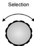
This rotary knob has no end stop. With every position **Selection(5)** selects another element in the display resp. another parameter in the setup menu. An arrow (->) is placed in front of the selected element/parameter.
