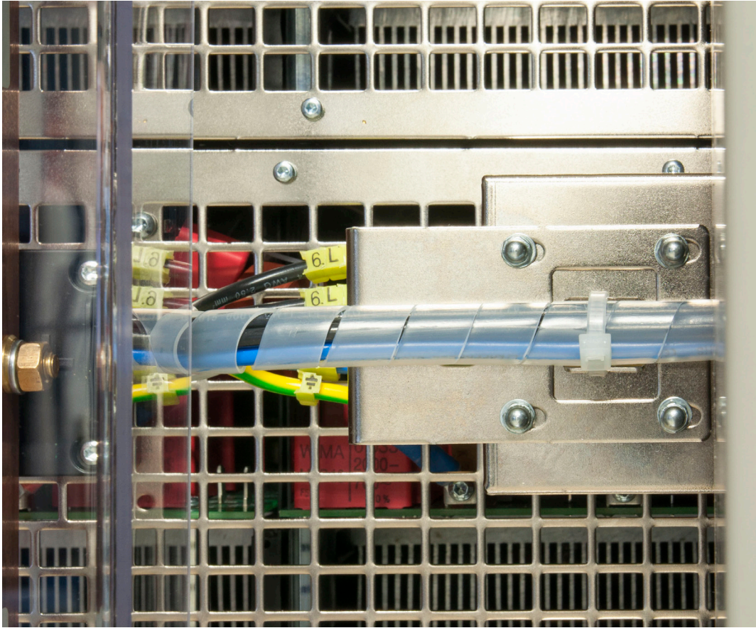
AC connection plug of the single units, with strain relief and fixing
