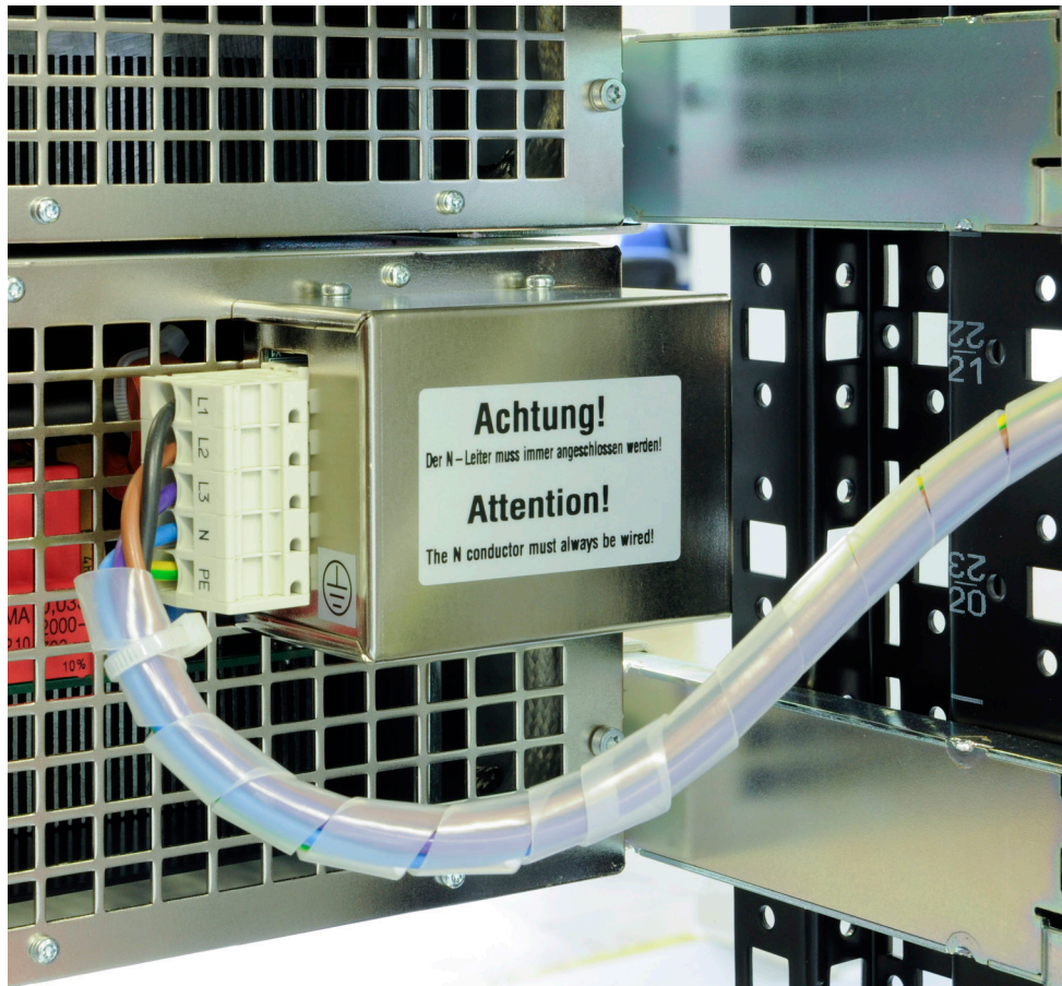
Figure 4 - AC input terminal of ELR/PSI units
