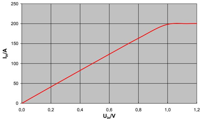
The curve between 0 and  $U_{\min}$  is linear so the current, that a certain model can take at even lower input voltages, can be calculated. Following  $U_{\min}$  are valid for  $I_{\max}$ :
