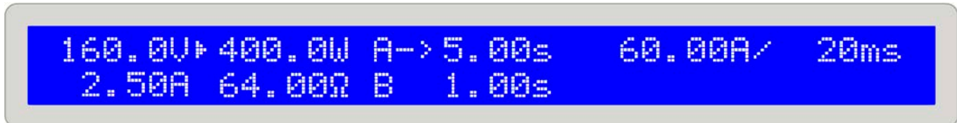
Figure 10. Level A/B operation with pulse width adjustment
