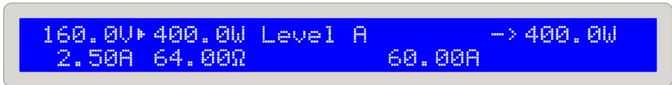
Figure 9. Normal load operation in CP regulation mode
