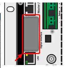
Figure 3 - Interface module slot
