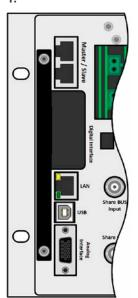
Remove the slot cover. If needed, use a screw driver.
