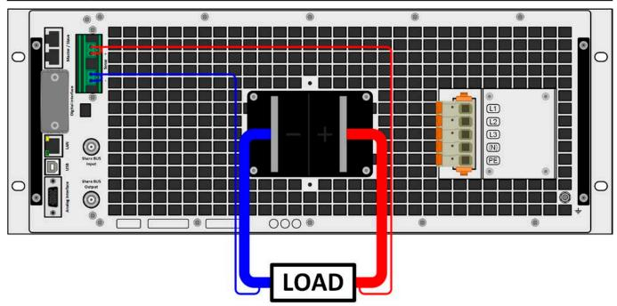
Figure 13 - Example for remote sensing wiring (DC terminal and Sense terminal covers left away for illustrative purposes)
