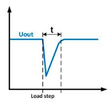
Example for a pos. load step: the DC output will collapse below the adjusted value for a short time. t = transient time to settle the output voltage.
