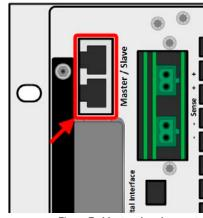
Figure 7 - Master slave bus ports
