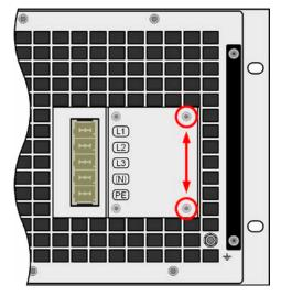
Figure 10 - Mounting position of the bracket
