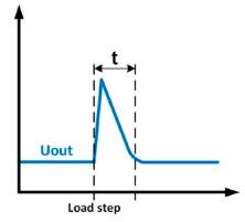
Example for a neg. load step: the DC output will rise above the adjusted value for a short time. t = transient time to settle the output voltage.
