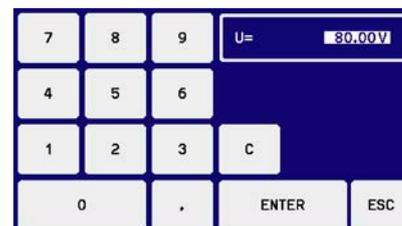
Decimal values are set by tapping the point key. For example, 54.3 V is set with **5** **4** **.** **3** and **ENTER**.
