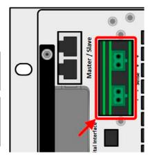
Figure 6- Remote sensing terminals
