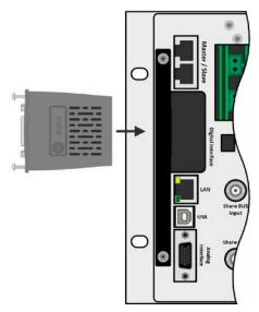
Insert the interface module into the slot. The shape ensures correct alignment.
