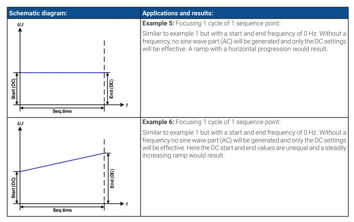
By linking together a number of differently configured sequence points, complex progressions can be created. Smart configuration of the arbitrary generator can be used to match triangular, sine, rectangular or trapezoidal wave functions and thus, e.g. a sequence of rectangular waves with differing amplitudes or duty cycles could be produced.
