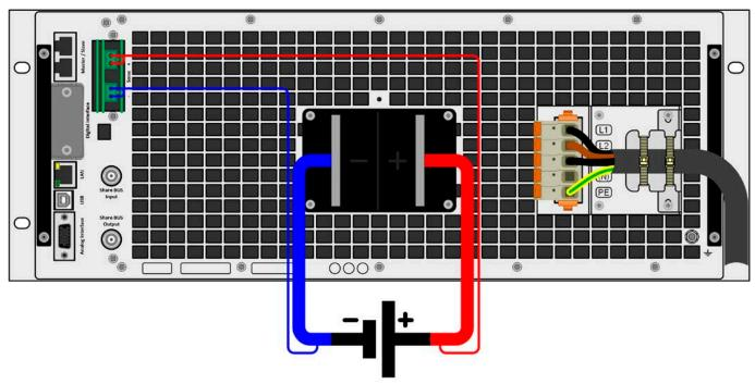
Figure 14 - Example for remote sensing wiring (DC terminal and Sense terminal covers left way for illustrative purposes)
