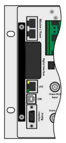
Remove the slot cover. If needed, use a screw driver.
