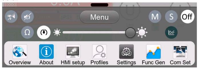
Tapping a button activates or deactivates the feature. Buttons with black on white indicate an activated feature:
