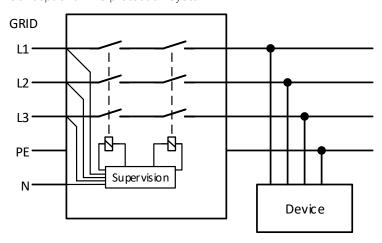
Figure 9 - Principle of an NS protection network
