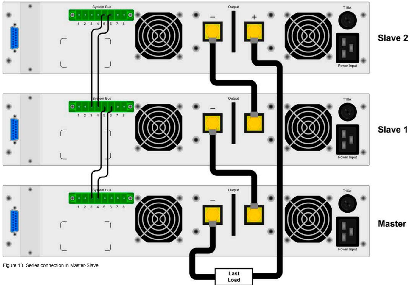
Figure 10. Series connection in Master-Slave
