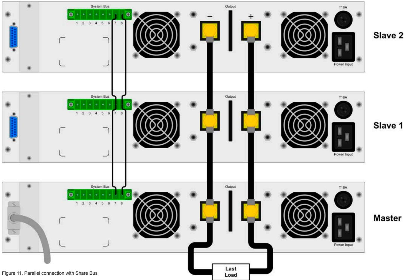
Figure 11. Parallel connection with Share Bus
