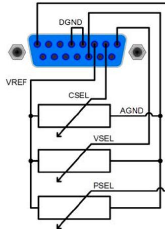
**Remote control of current and voltage**
