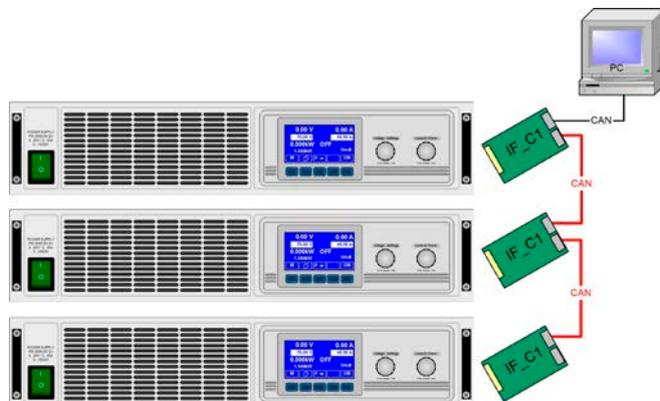
Figure 13. CAN networking example, also applies to GPIB
