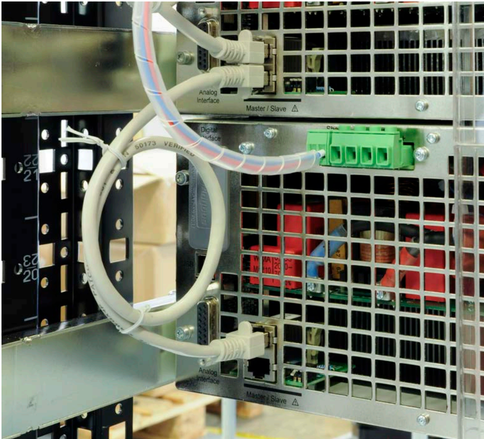
Figure 5 - Master-slave and Share bus wiring
