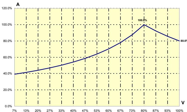
Bild 9 - Derating curve of linear ACP models
