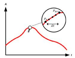
With interpolation - the curve remains linear
