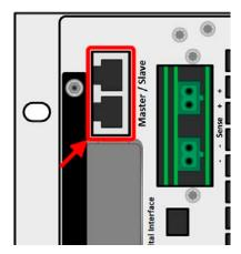
Figure 7 - Master slave bus ports
