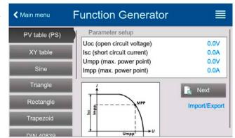
• the maximum power point (MPP), at which the solar panel can provide the maximum output power, defined by  $U_{MPP}$  and  $I_{MPP}$
