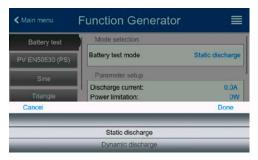
There is a choice of modes: **Static discharge** (constant current), **Dynamic discharge** (pulsed current), **Static charge** (constant current) and **Dynamic test** (flow of charge/discharge).
