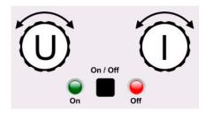
The physical quantities on the depiction of the knob show the current assignment. The left knob is always assigned to the voltage (U), while the right knob can be switched by tapping on the depiction. Furthermore, the DC terminal status is indicated by two LEDs (green = on).
