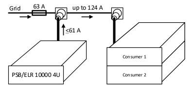
When running a higher number of recovering, i. e. energy backfeeding units on the same leg of the installation, the total currents per phase increases accordingly.
