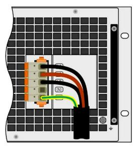
Figure 10 - Example for an AC cable with 4 conductors (european color code, cable not included in delivery)
