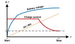
The fourth mode is called **Dynamic test** and combines **Static discharge** with **Static charge** in one flow. The same parameters for the single test parts are available, plus some extra for the flow. You can, for example, select what comes first, charge or discharge. There is also an option to cycle the test, i. e. repeat 1 to 999 times or infinitely and you can define a resting period which elapsed before the next cycle.
