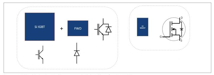
Figure 11. Si IGBT and diode pc board pad layout compared with the pad layout for a SiC MOSFET
