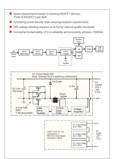
Figure 5. Si transistor-based 5 kW power module which uses three Si MOSFETs
