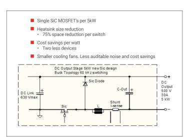
Figure 13. SiC transistor-based output stage enabled a 45% increase in power density.
