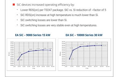
Figure 14. Improvement in efficiency over the power output range of the new 10000-series supplies compared with the older generation 9000-series supply.
