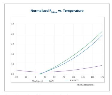
Figure 7. Comparison of  $R_{\scriptscriptstyle DS(on)}$  as a function of temperature among a SiC MOSFET, a GaN MOSFET, and a SI MOSFET
