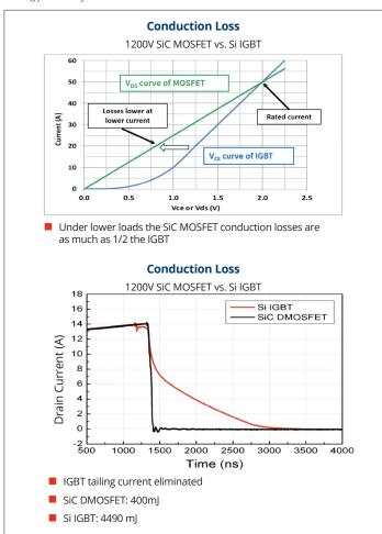
Figure 6. Comparison of switching and conduction losses between a SiC MOSFET and a Si IGBT
