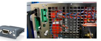
Figure 6. Anybus communication interface modules (on the left) are easily installed into an EA power supply's digital interface slot (on the right) and can be swapped based on changing test needs with a simple screwdriver.
