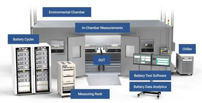
Figure 2. Typical lab setup for battery validation.
