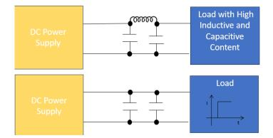
Figure 4. (Top figure) A Pi filter can isolate the power supply from high-frequency effects.
