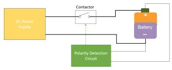
Figure 3. A polarity detection circuit controls a contactor to prevent applying power to a battery if the battery has been incorrectly connected into the circuit.
