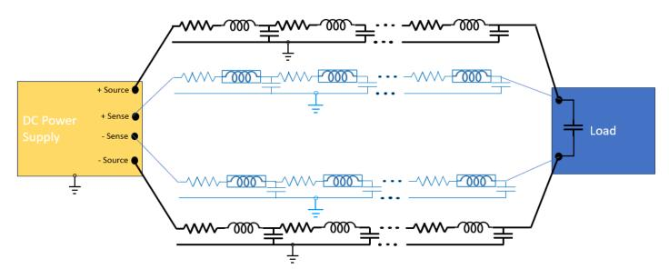
Figure 6. A power supply-load circuit with the source and sense lead wires represented as distributed R-L-C networks. Even though the power supply is delivering DC voltage, the circuit is essentially an AC network.
