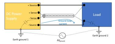
Figure 8. Noisy ground current enters the sense circuit when the DC power supply and load are at different voltages.
