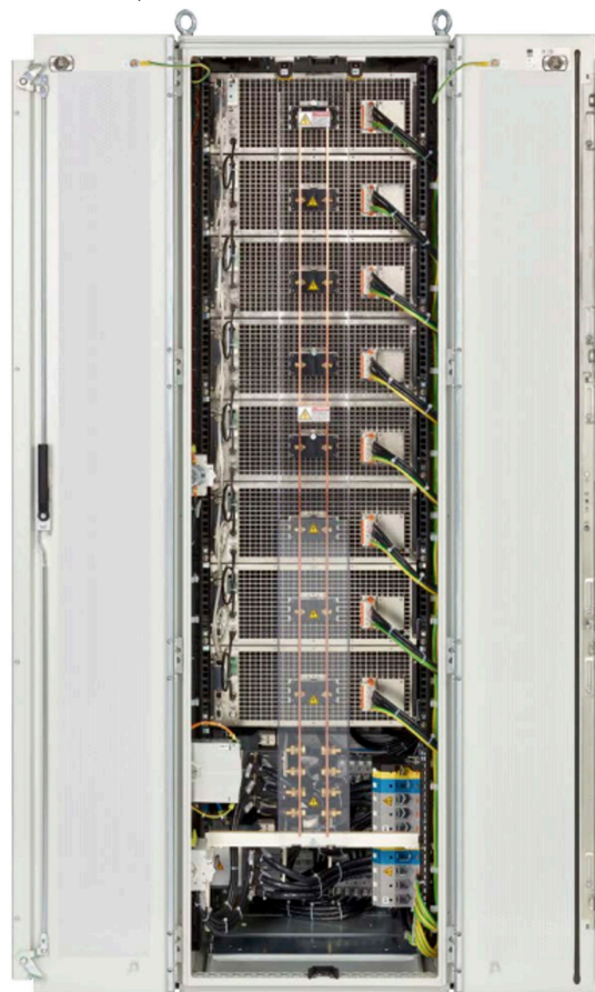
Figure 3. Rear of a 240 kW test rack showing the simplified wiring designed for maximum safety and reliability
