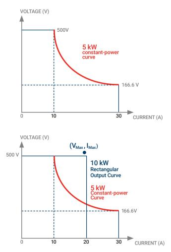
Figure 2. The autoranging characteristic of EA power supplies compared with a higher power rectangular output power supply.
